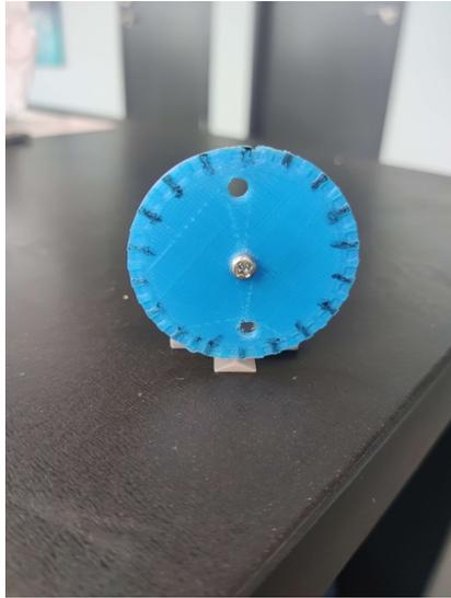
(a) Jig used to keep the two ends of the differential pressure sensor probes 3 cm apart while rotating during experiments.
