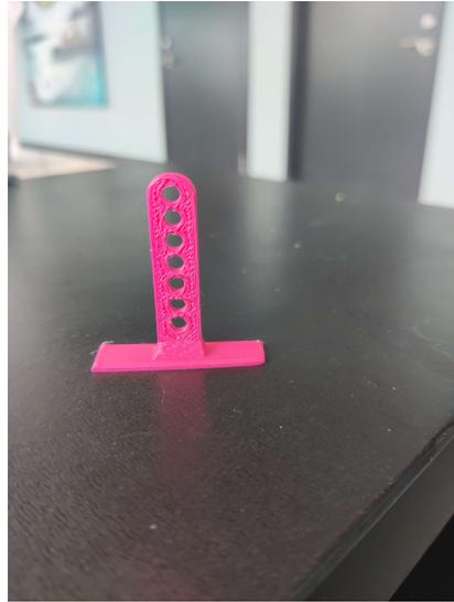
(b) Spacing jig used to keep the two ends of the differential pressure sensor probes 3cm apart during experiments.
